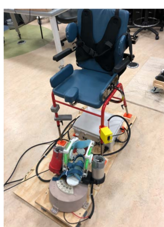
Left: Pedbot with 3 DOFs: pitch (dorsiflexion and planterflexion), roll (eversion and inversion), and yaw (abduction and adduction). Center: Child with cerebral palsy (a) playing airplane video game using PedBot as an input device (b). Photograph used with consent of the parents and child. Right: PedBotHome System showing blue chair, control box under chair, and device in front with smart phone under foot plate (not seen).
