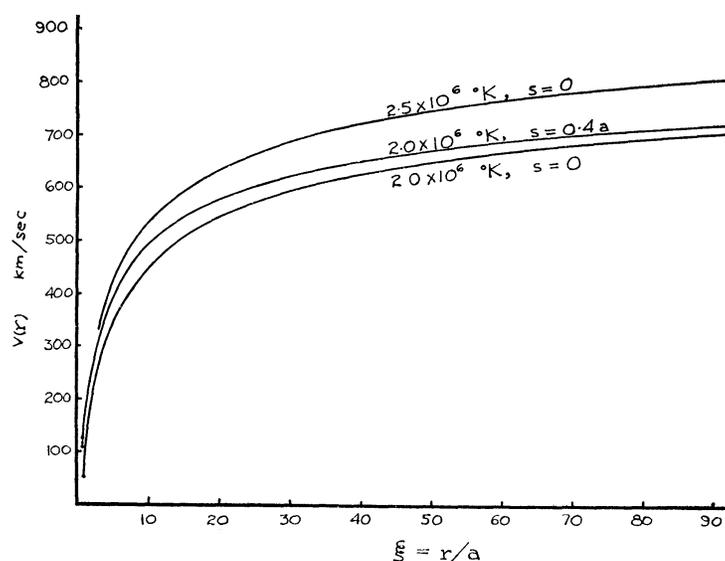
FIG 3—Hydrodynamic expansion velocity outward from a point distant  $0.4a$  from the center of the sun with a coronal temperature of  $2 \times 10^6$  °K, compared to expansion with spherical symmetry about the center.
