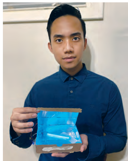
Marshall Mendoza designed the “De-Colonizer 7000” to clean face masks using UV light
