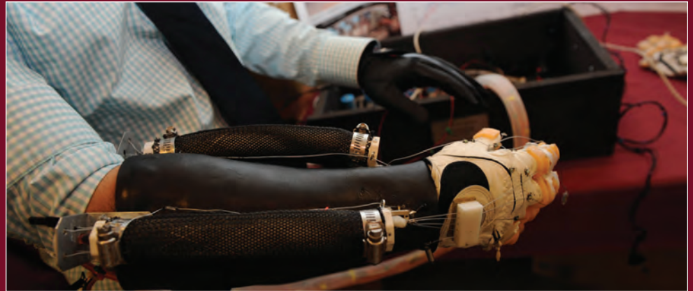
Hand Assistive Rehabilitation Pneumatic Exoskeleton (HARPE).
